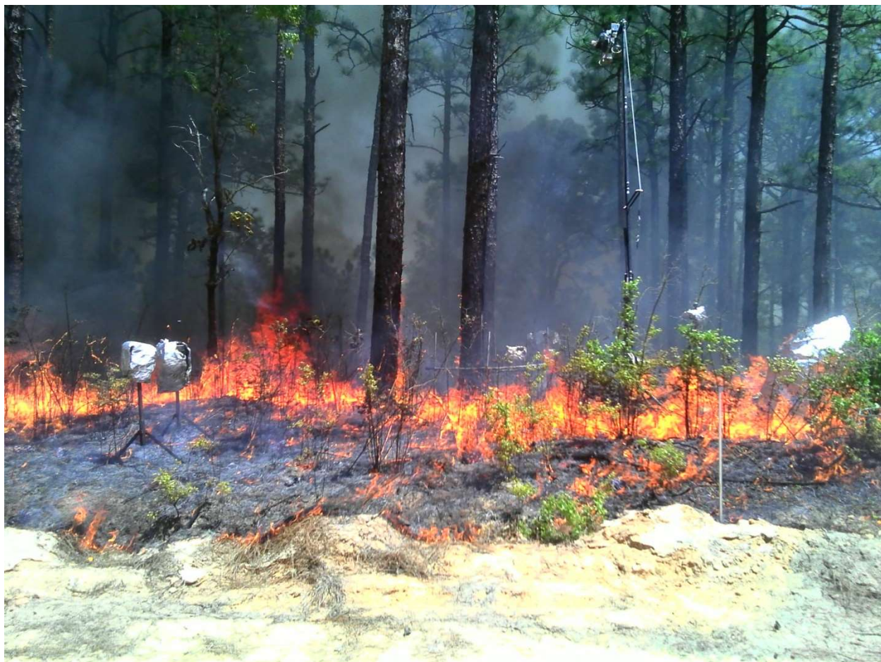
Figure 7 Fire behavior in the reference plots of burn 4. Instruments registered a peak total heat flux of 19.3\text{ kW/m}^2 , a peak air temperature of 714^\circ\text{C} , and a peak horizontal wind speed of 3.6\text{ m/s} .
