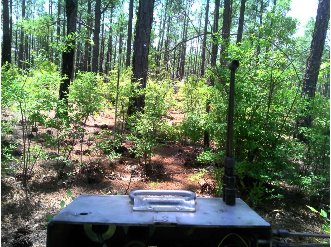
Figure 11 Fuel loading for plot 7. A peak total heat flux of 17.8\text{kW/m}^2 was registered along with a peak air temperature of 930^\circ\text{C} and peak horizontal wind speeds of 4.3\text{m/s} .
